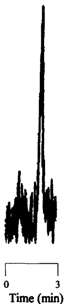
Fig. 10. Peak resulting from flow injection of 1.40 ppm nitrogen of indole via a 5- \mu l sample loop with a split ratio of 1/116.5 (CLND/UV). Minimum detectable quantity is 60 pg nitrogen at S/N=3 .
